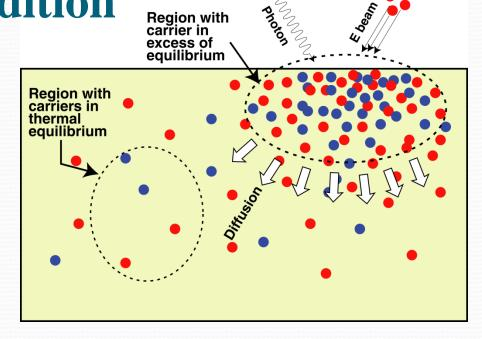
Obviously not. Because the carriers recombine and as it expands, the gradient is smaller and the diffusion is weaker. Intuitively, the harder we pump, the bigger the EH gas volume should be. How do we describe this quantitatively?
